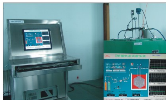
O-ring explosion-proof test
