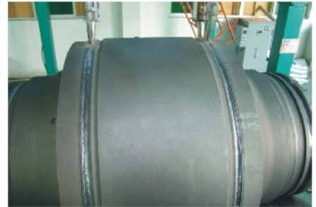
Ultrasonic weld testing
